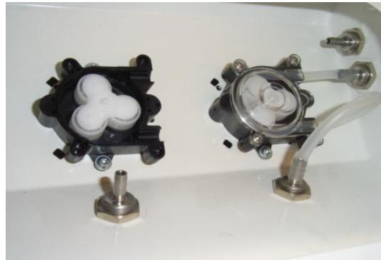
Remove the old hose from the metal hose connector and take it out of the dosing head.
