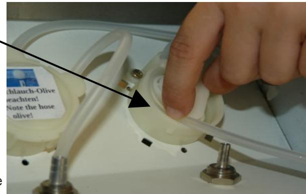
Clip on the pump cover and attach the hose to the lower metal connector at an even arc onto the metal connector.
