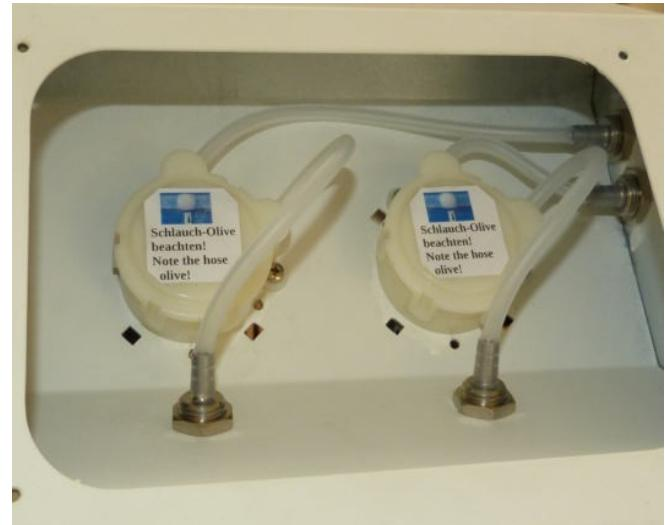
To replace the dosing hose, the dosing pump head must be opened. To do this, unclip the 4 cover retaining tabs from their locks, starting with the tab between the hoses, then continue in sequence. Use a small screwdriver if necessary.
