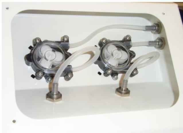
To replace the dosing hose, the dosing pump head must be opened. To do this, unscrew the 4 Phillips screws on the mounting eyelets on the transparent cover and remove the transparent cover.
