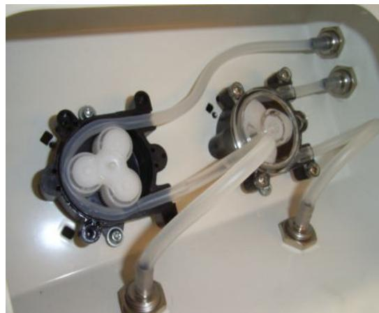
Put the transparent cover on and carefully tighten the screws. Attach the end of the hose to the lower metal connector in a smooth arc.
