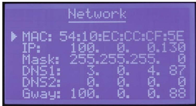
After connecting the system to the company network, the ÖKO 2000 obtains an IP address via the DHCP system.
