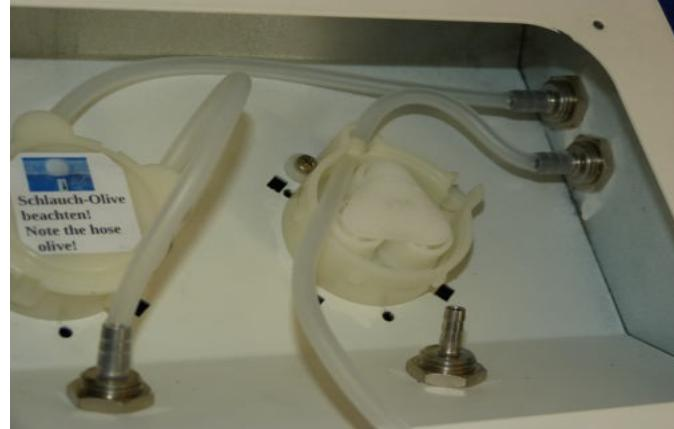
Continue inserting the hose into the pump ahead, turning the rollers counterclockwise and guiding the hose into the housing.
