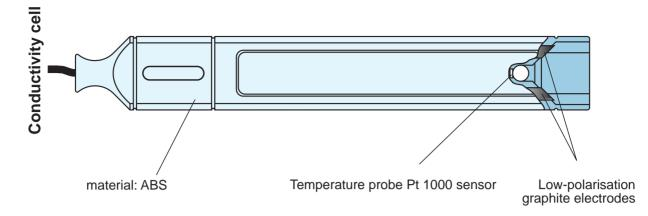
**Warning:** Conductivity cell is only operatable in watersoluble mediums, otherwise measuring contacts will be affected and therefore results will be wrong!
