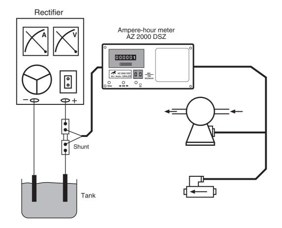
The dosing System DSZ causes a timer to be started up at intervais of 10 / 100 or 1000 Ah/Amin.
